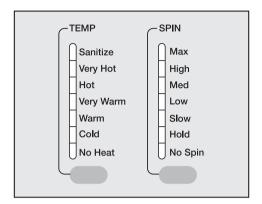
Press the "TEMP" and "SPIN" buttons until the indicator of the desired value lights.
